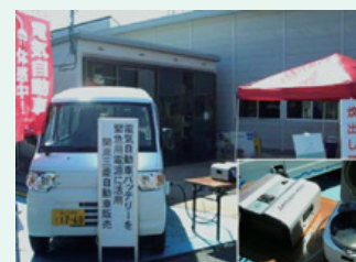
Supplying power to a rice cooker (during a disaster drill in Kawasaki)
