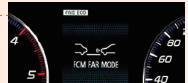
Forward Collision Mitigation System lamp within combination meter
